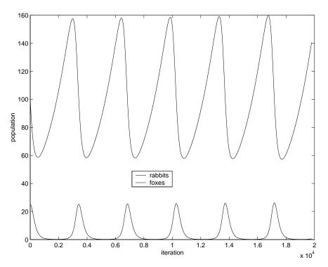
**FIGURE 6.7:** Simulation of preditor prey equations. We have selected the initial conditions  $f_0 = 25$  and  $r_0 = 100$ . In addition the parameters were chosen to be  $g_1 = .01, g_2 = .0005, c_1 = .0001, c_2 = .0001, d_1 = 0.0, d_2 = 0.0$
